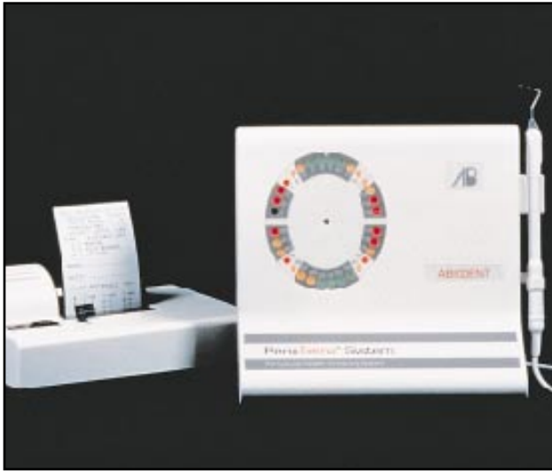
Figure 1. Automated periodontal probe detects temperature changes associated with inflammation in the gingival sulcus (PerioTemp, Abiodent, Danvers, MA). (Used with permission of Abiodent.)
