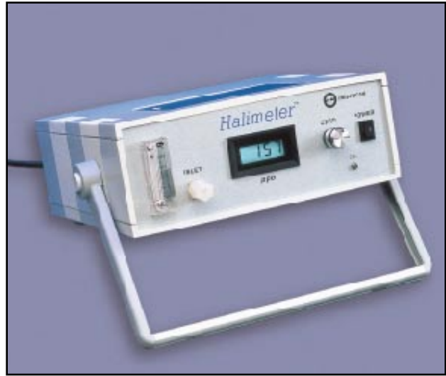
Figure 2. Portable sulfide monitor, calibrated with hydrogen sulfide and measured in parts per billion (Halimeter, Interscan Corporation, Chatsworth, CA). (Used with permission of Interscan Corporation.)
